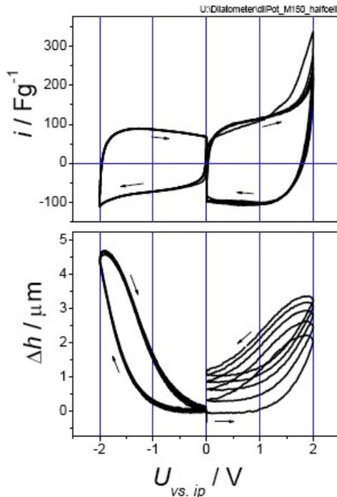
**Figure 3:** Top: EDLC half cell CVs (1st to 5th cycle) for the extended negative (0 to -2 V) and the extended positive potential range (0 to 2 V). Scan rate: 10 mV/s. Bottom: Simultaneous dilatation record. 1M TEABF<sub>4</sub> in AN, activated carbon.
