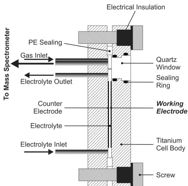
**Figure 1:** MS cell used for headspace analysis of the gases evolved during cyclic voltammetry.
