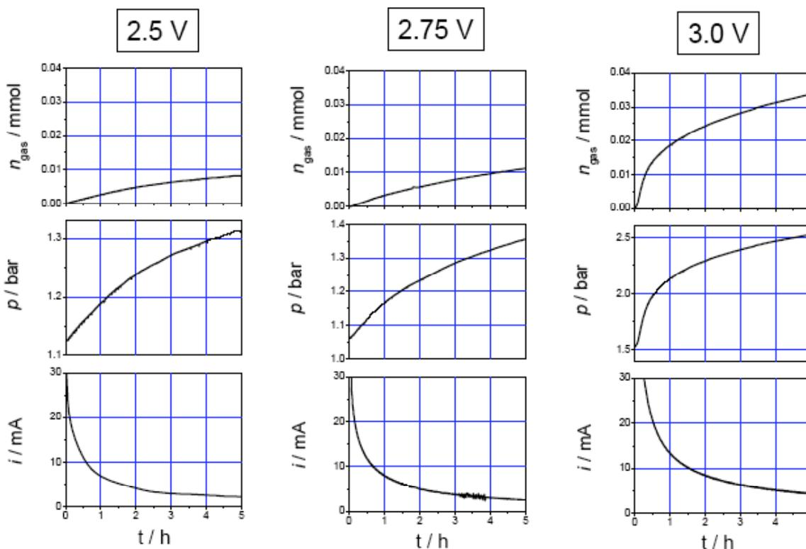
**Figure 5:** Pressure increase as a function of time monitored at constant cell voltages of 2.5 V, 2.75 V and 3.0 V. 1 M TEABF<sub>4</sub> in PC
