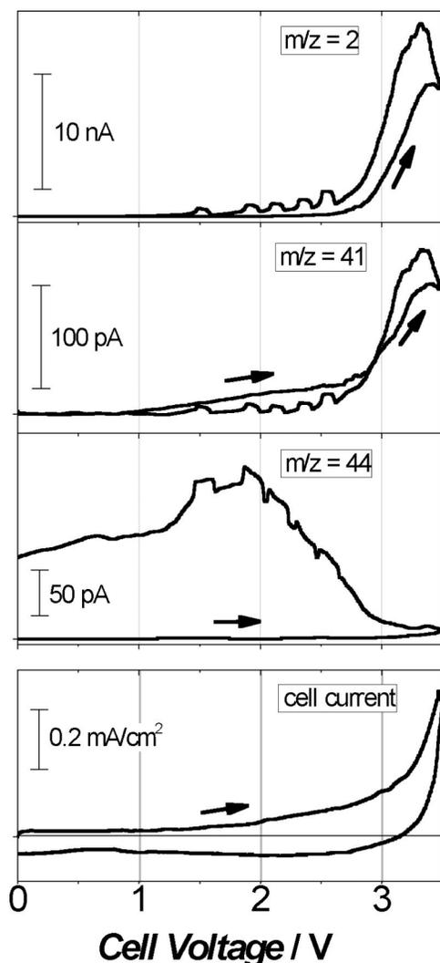
**Figure 4:** First cycle of the CV (bottom) and simultaneous gas evolution as detected by on-line mass spectroscopy (MSCV). The set-up used is shown in Fig. 1. Scan rate: 0.1 mV/s. 1M TEABF<sub>4</sub> in PC.
